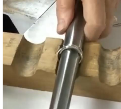
Gently hammer the metal strip into a swag to shape the ring; screen shot OLMC Silversmiths 2022-03-22
