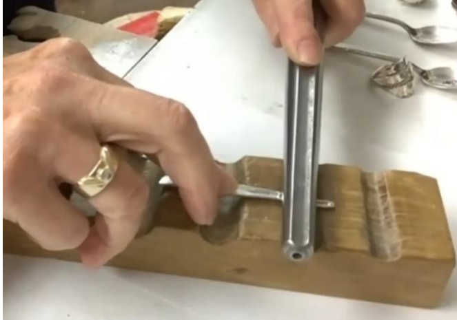
Gently hammer the metal strip into a swag to shape the ring; screen shot OLMC Silversmiths 2022-03-22
