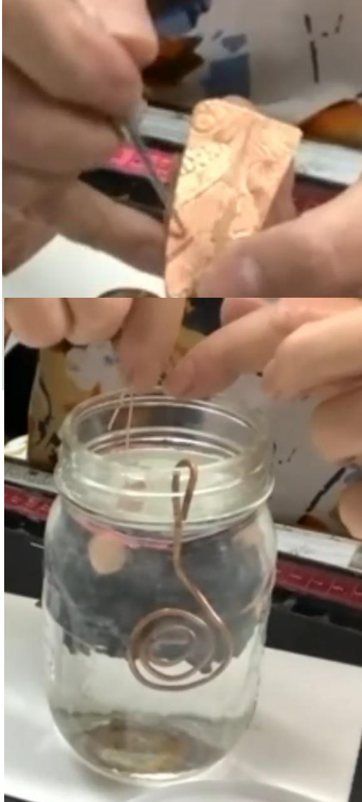
Etch a design in the metal piece. Then immerse it into a prepared salt water solution, across from a looped wire that will be electrified.
